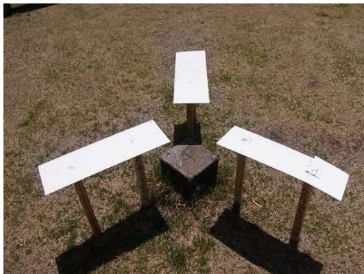
Ground Control Point (GCP)
